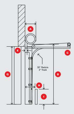
NOTES: A torsion bar support is required on all doors 10' or wider. The Rasco door has outside pull brackets/cables.
