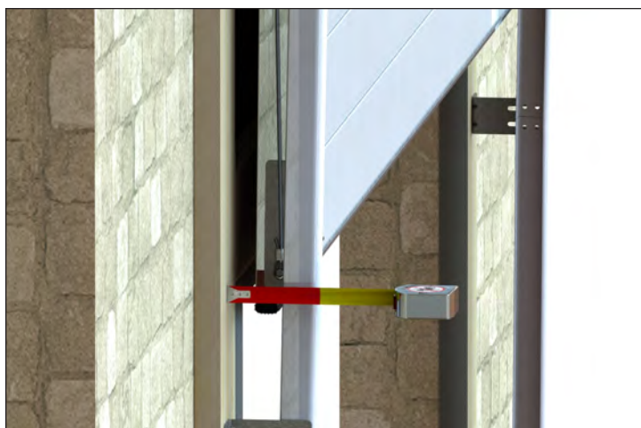
3 Distance from wall to furthest part of existing track at top of the opening To ensure a proper seal on the sides, many tracks are farther away from wall at top of opening.
