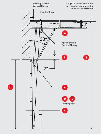
**NOTES:** A torsion bar support is required on all doors 10' or wider. Switch track cannot be used if existing door has outside pull cables or has TKO, Workhorse or Barcol type tracks. The Rasco door has outside pull brackets/cables.
